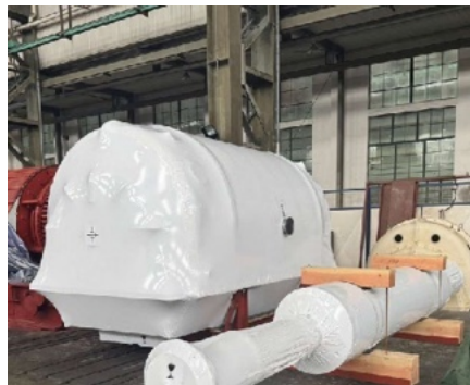
GT3 GE Frame 6B Gas Turbine Generator Package — Full enclosure and auxiliary systems
