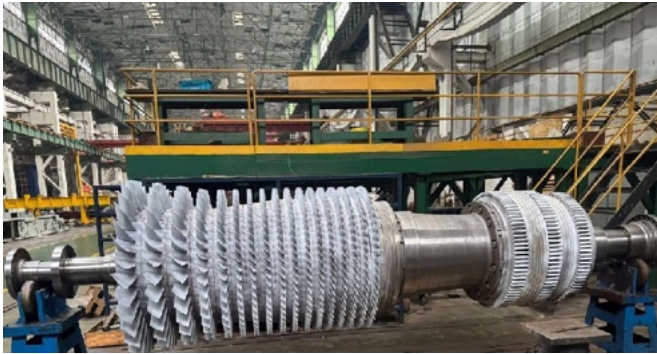
GE Frame 6B Compressor Rotor
